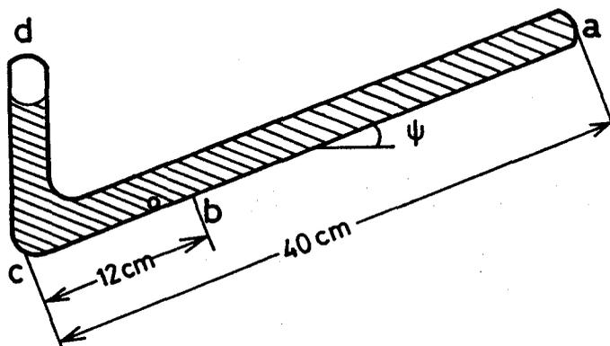
Figure III-1. Schematic diagram of a rolling-ball viscometer.
