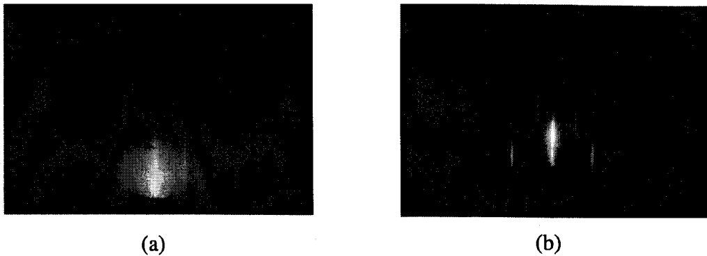
Fig. 3-4 RHEED patterns of Pt thin thin films on (a) annealed and (b) non-annealed (100)MgO. \langle 100 \rangle azimuth.
