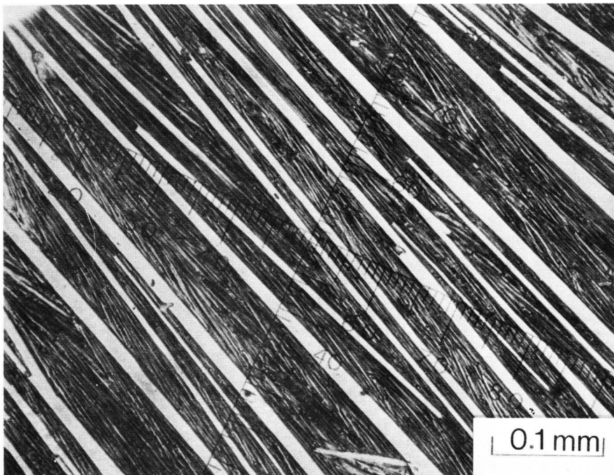
Fig. 61. Microstructure of mixture containing 0.6 mass fraction of \text{CO}(\text{NH}_2)_2 .
