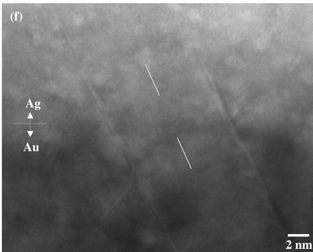
Fig. 4-14 TEM images of cross-sections of bonds with silver or gold plating: (e) and (f) high-resolution images (Ag/Au).
