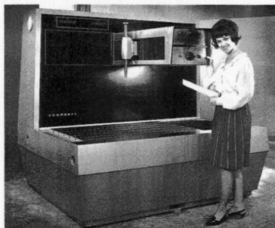
Figure 1.4: First coordinate measuring machine by Ferranti [62].
