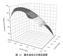
Fig. 12 Experimental result of fundamental component.
