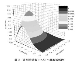
Fig. 8 Fundamental coefficient of tandem EAM.
