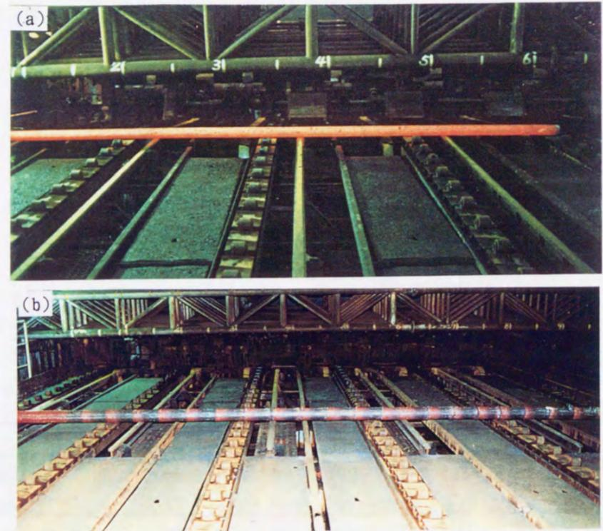
(a)no obvious defects (b)cracks in longitudinal direction
