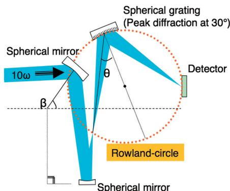
Fig. 2 Overview of setup of Rowland-type spectrometer.
