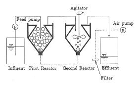
Fig. 2 Schematic diagram of experimental apparatus for experiment III
