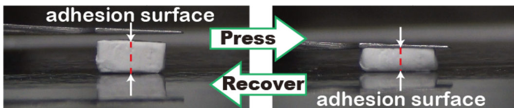
Figure 2-8. Self-healing behavior observed by press test. Healed samples can sustain large deformations. Although scars are not visible, repaired samples break at joints, expect when allowed to heal for a long period.
