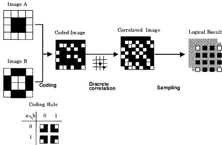
Fig. 3 Processing procedure of optical array logic.
