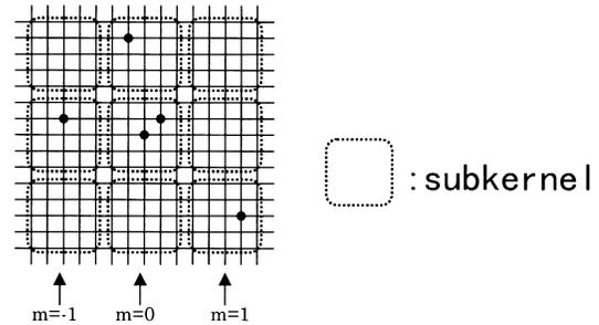
**Fig. 5** Division of correlation kernel.
