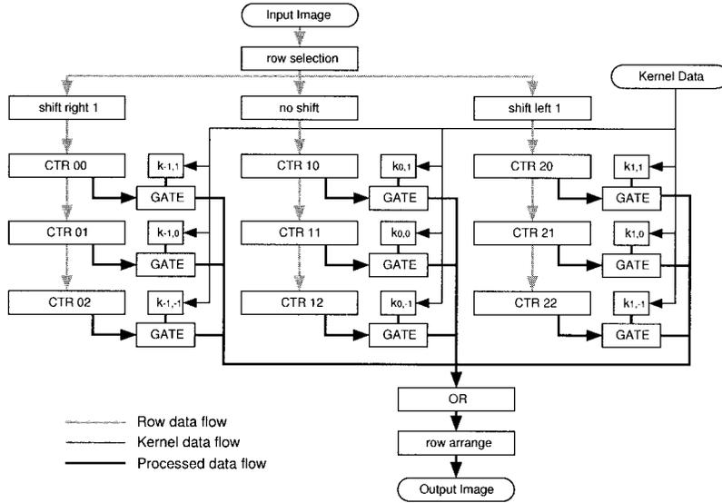
Fig. 7 Block diagram of the PDC.
