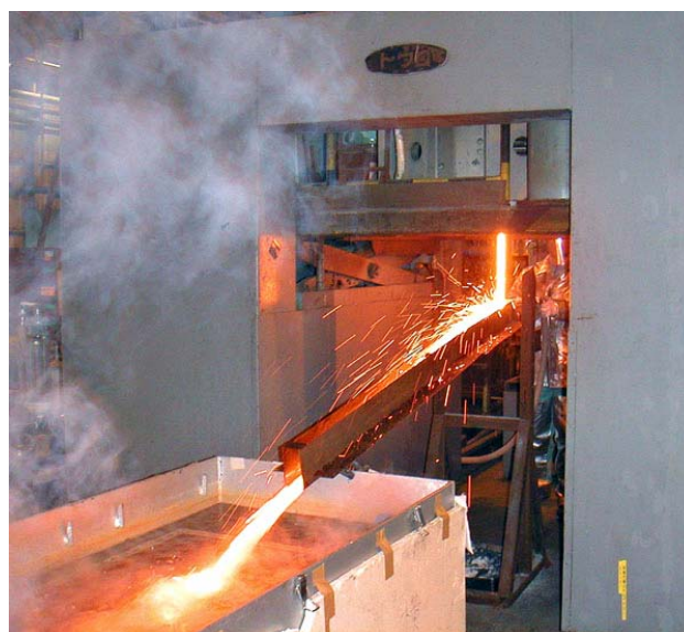
Fig. 3-4. View of laboratory scale water granulation experiment.
