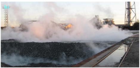
Fig. 2-4. View of air cooling blast furnace slag in slag cooling yard.a) Poring from slag ladle. b) Water cooling.
