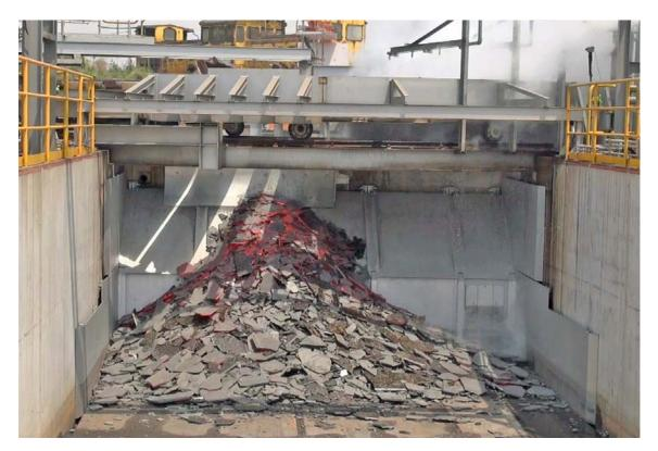
Fig.2-56. Solidified slag with PACSS®.
