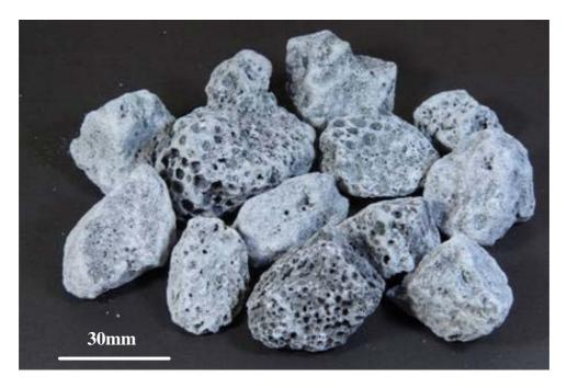
Fig. 2-1. Appearance of air cooled blast furnace slag.
