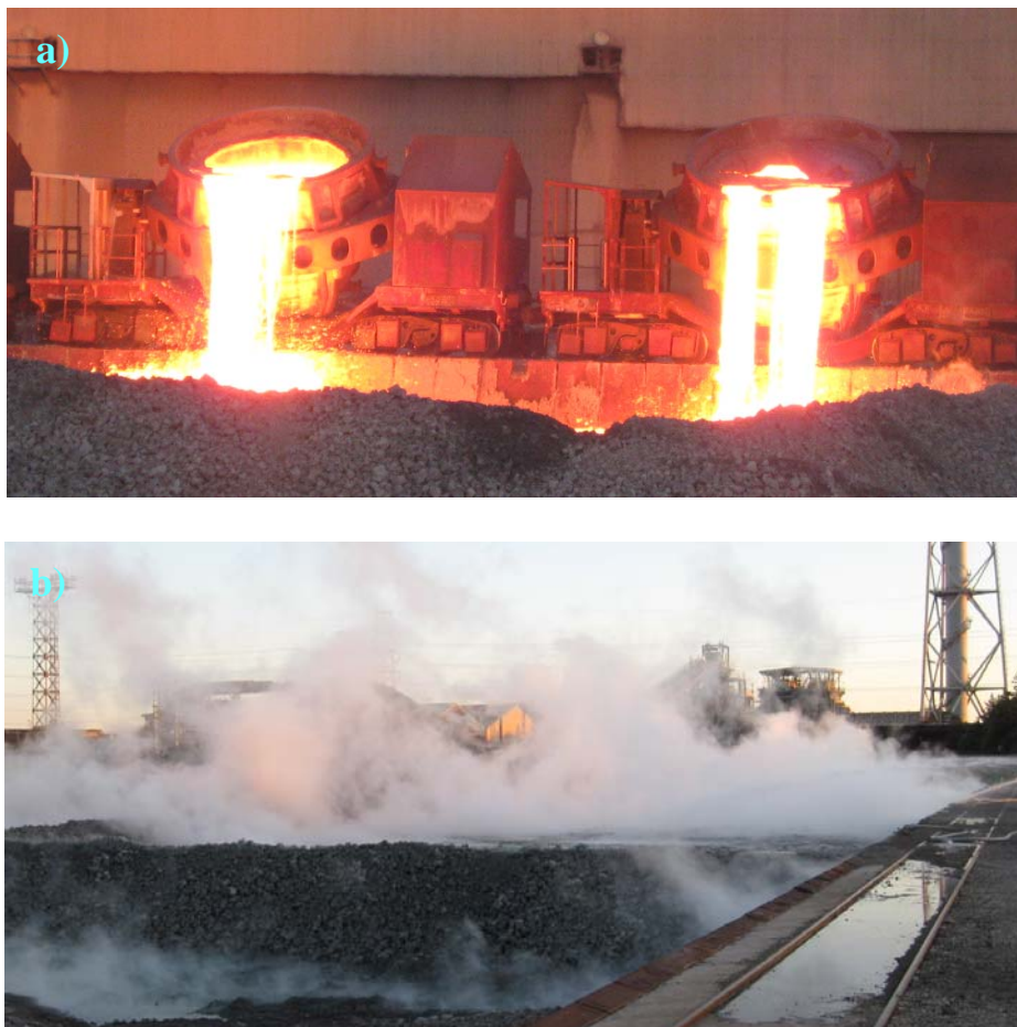
Fig. 2-4. View of air cooling blast furnace slag in slag cooling yard.
