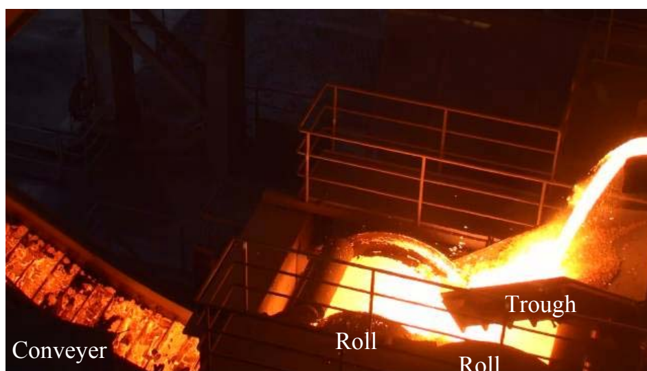
Fig. 4-21. View of pilot experiment by twin roll type continuous slag solidification process.
