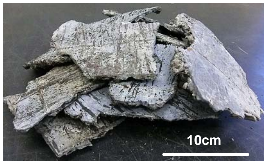
Fig. 4-24. Appearance of solidified slag after twin roll process.
