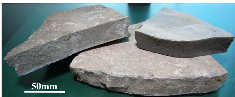
Fig. 2-39. Appearance of plate-like solidified slag with pilot plant.
