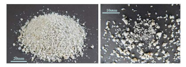
Fig. 1-5. Water granulated blast furnace slag.
