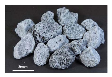
Fig. 1-7. Air cooled blast furnace slag.
