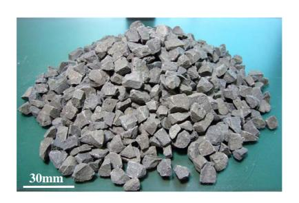
Fig. 2-42. Appearance of crushed aggregate made from plate-like solidified slag.
