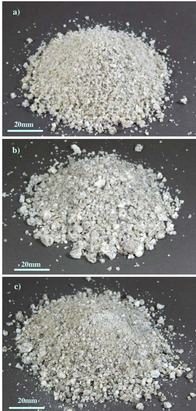
Fig. 3-32. Appearance of water granulated slag. a) Conventional water granulated slag for blast furnace cement. b) Developed water granulated slag for fine aggregate. c) Coarse fine aggregate after grinding developed water granulated slag.
