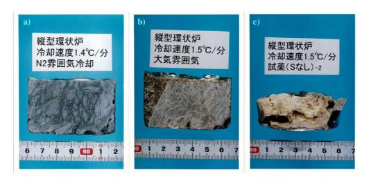
Fig.2-27. Effect of atmosphere and sulfur content on pore generation.
