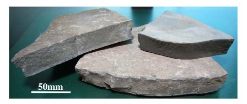
Fig. 2-39. Appearance of plate-like solidified slag with pilot plant.
