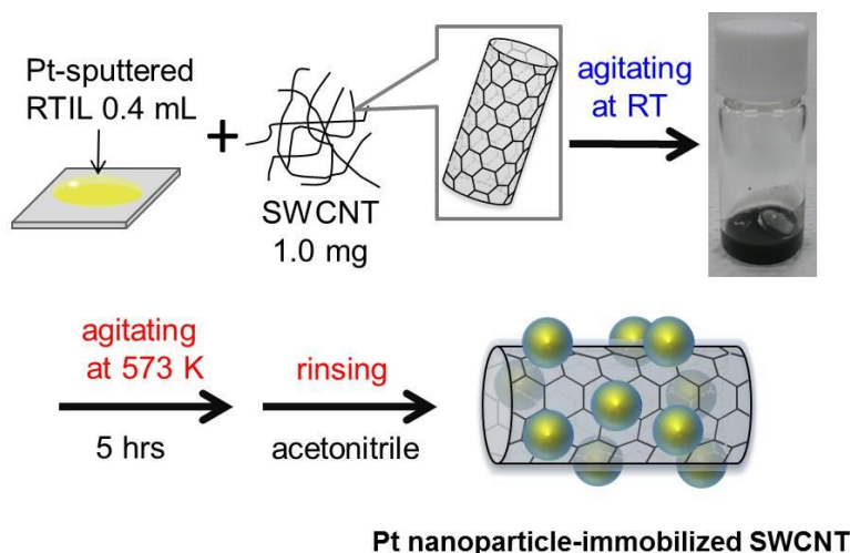
Scheme 2-1. Fabrication method for Pt nanoparticle-immobilized SWCNT composite material used in this investigation.
