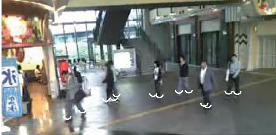
Figure 5.2 Pedestrian walking in a shopping mall. The white marks represent the detected feet of pedestrians. Motion of each pedestrian is observed using wearable accelerometer and LRFs by tracking each foot.
