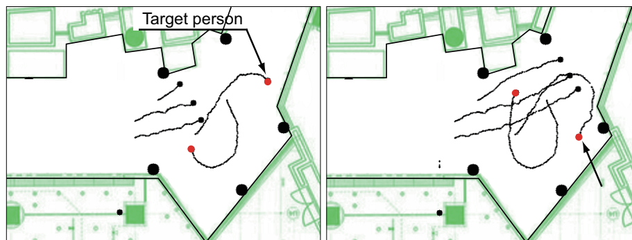
a) Observed trajectories using LRFs
