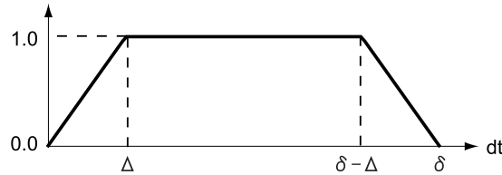
Figure 3.12 The probability that steps of two people are separately observed when the time difference of the steps is dt . \Delta represents the sampling period, and \delta represents the period of walking steps. This figure shows the case \Delta < \delta/2 .
