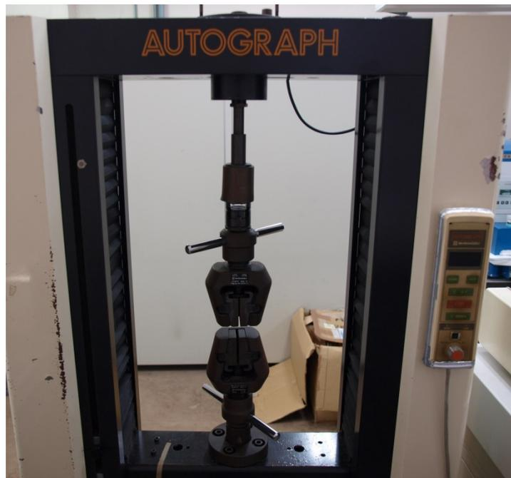
**Fig. 2.21** General views of tensile test machines used (AG-10Kne).
