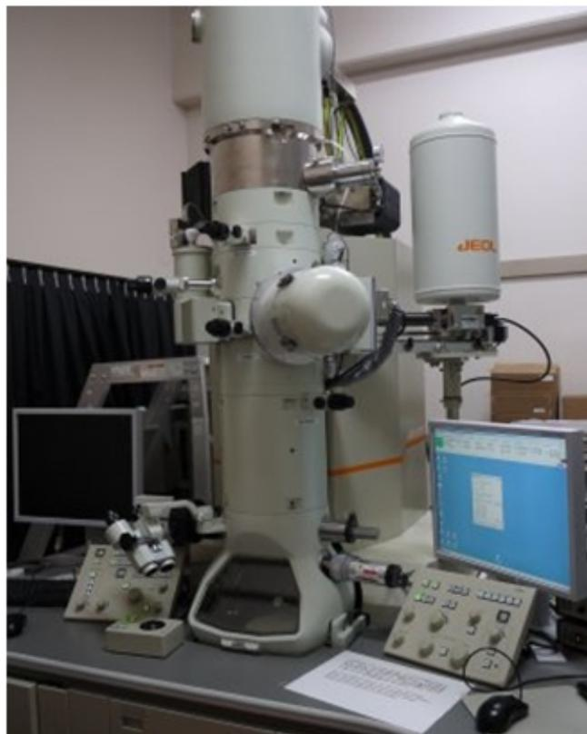
**Fig. 2.19** General view of transmission electronic microscope (TEM).
