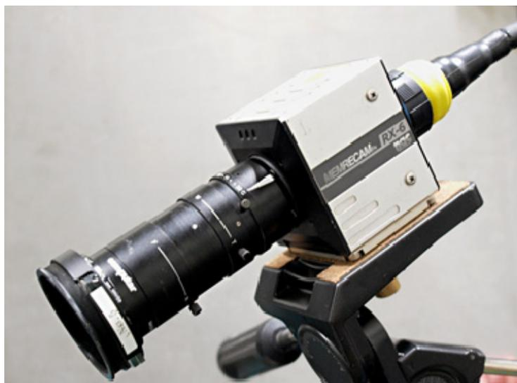
(a) General view of high speed video camera (MEMRECAM fx Rx-6)
