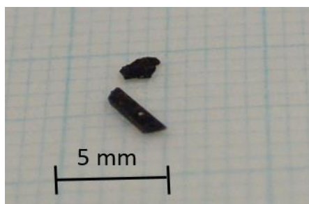
Figure 2-2: Obtained single crystals of Cr 2 O 3 by the flux method.
