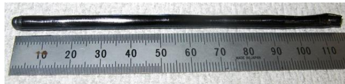
Figure 2-1: Obtained single crystal of \text{SmMnO}_3 by the floating-zone method.
