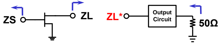
ZL*: Complex conjugate optimum load impedance Minimize the return loss measured from system port
