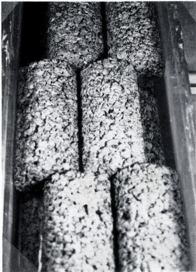
Photo 2.Setting condition of porous concrete in the 1st water channel.
