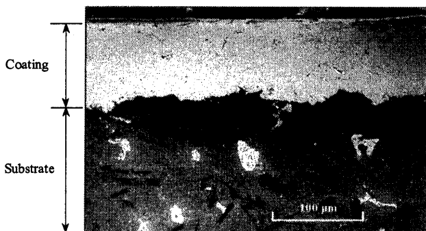
Fig. 1 Representative spray coating section with newly-developed powder.
