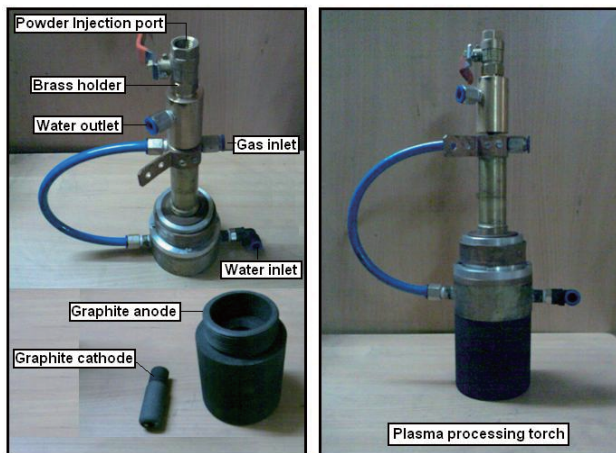
Fig. 1(b) Photographic images of electrodes and HCP torch.
