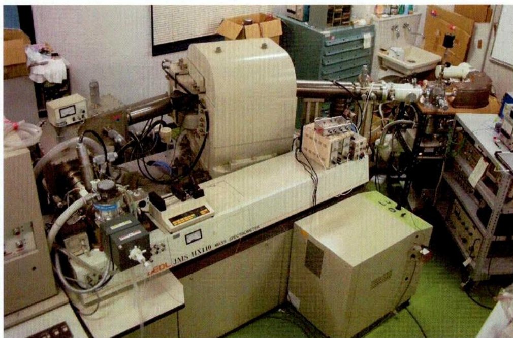
Fig. 4.5.2. Photograph of the MS/MS instrument equipped with quadrupole doublet lens.
