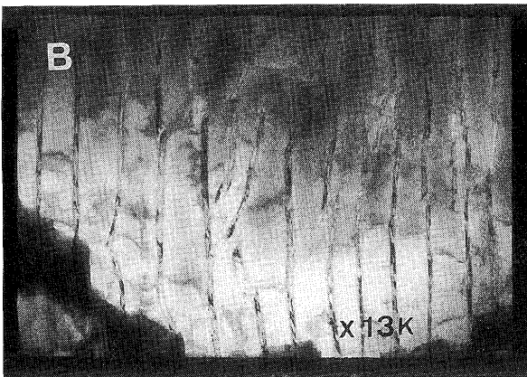
Fig. 6 SEM(A) and TEM (B) micrographs of nitrides
