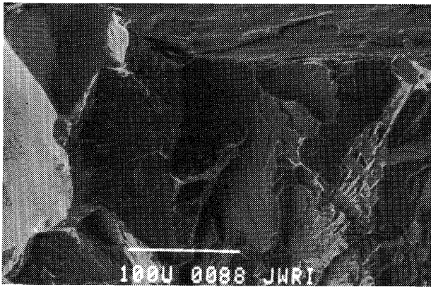
Fig. 9 Fracture surface of the impact specimen of the steel HT100-B after heat treatment 823K/4hr
