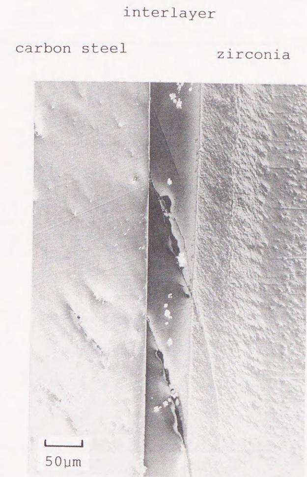
Fig. 3.5 Optical micrograph of the interface using borate solder (B5) joined at 1173K for 1.8ks.
