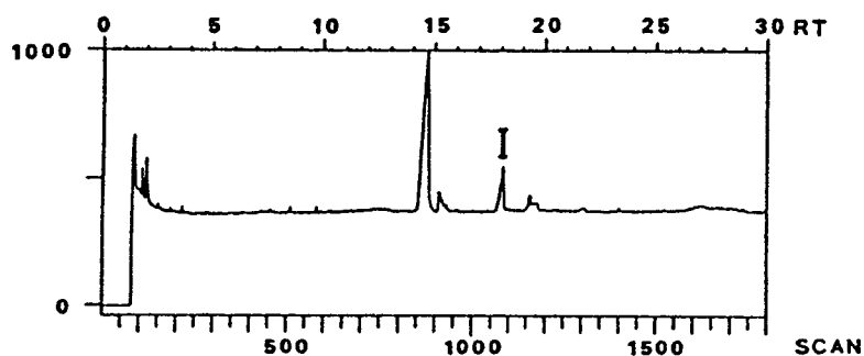
Fig. 1-4-2. Typical Total Ion Chromatogram of a Urine Sample of a Subject Acutely Poisoned with p -CNB by GC/MS under Condition-1.
