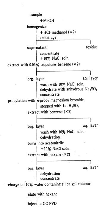
Chart 1. Schematic diagram for the analysis of mono-, di- and tri-*n*-butyltin compounds in rat tissues.
