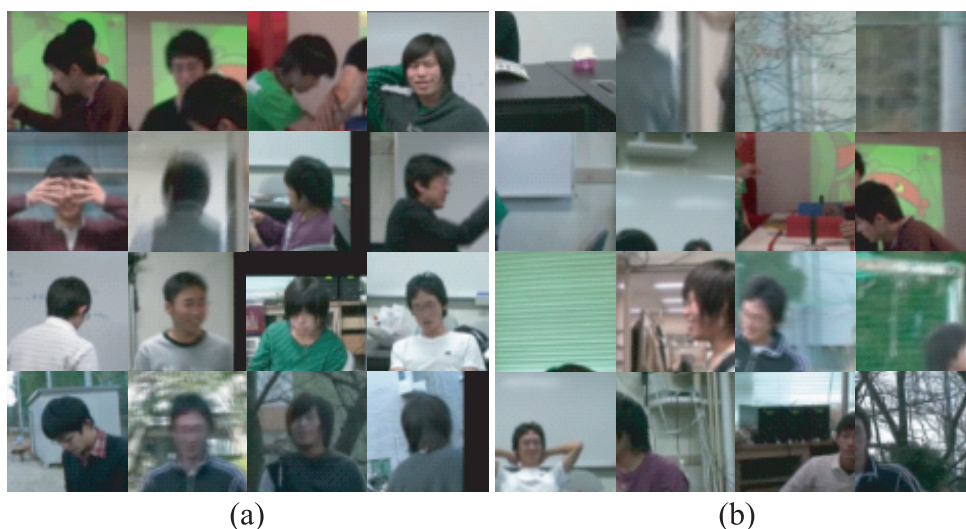
Figure 4.3: (a) Positive and (b) negative samples used to train support vector machine (SVM) for human object detection.
