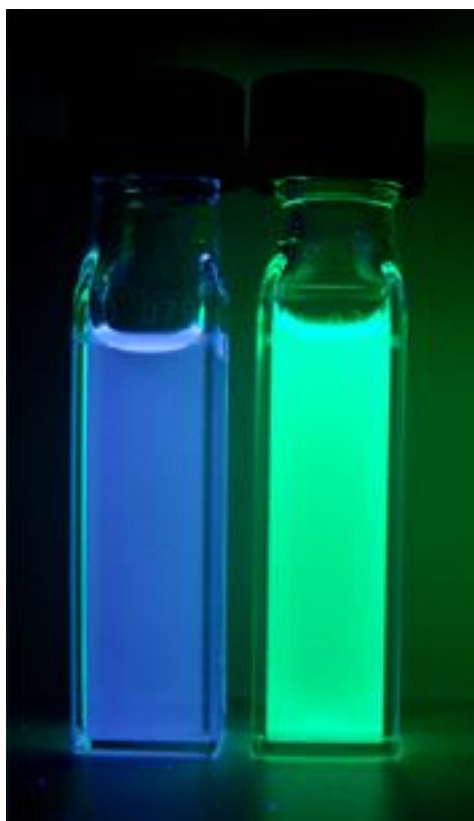
Figure 2-2. CdS NCs dissolved in NH 3 aqueous solution.
