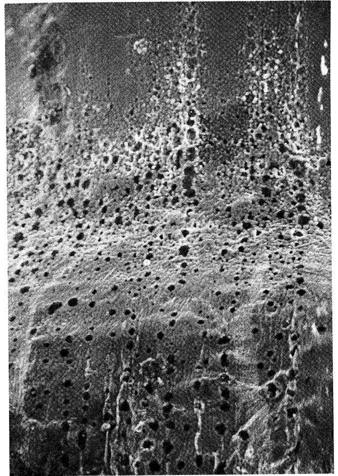
Fig. 9 Traces representing evaporation of wire materials due to climbing up of arc roots. (x 400)
