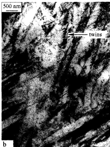
Fig. 4: Transmission electron micrographs of weld C. (a) Shows the expected mixture of bainitic ferrite plates interspersed with retained austenite films. (b) Region containing high-carbon, untempered martensite.
