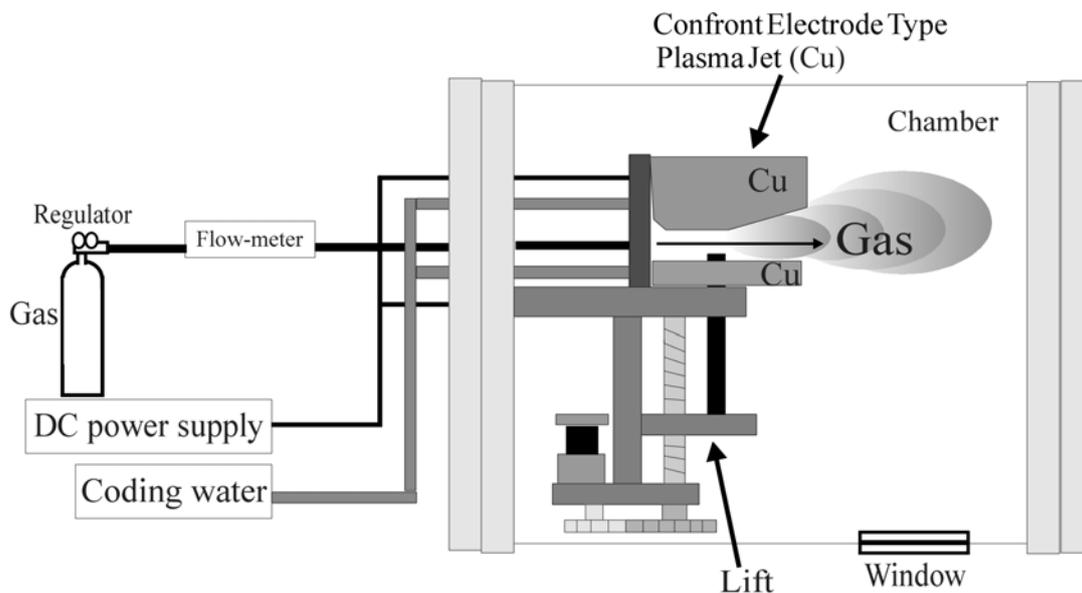
Fig.7 Schematic diagram of the movable confront electrode type plasma jet.
