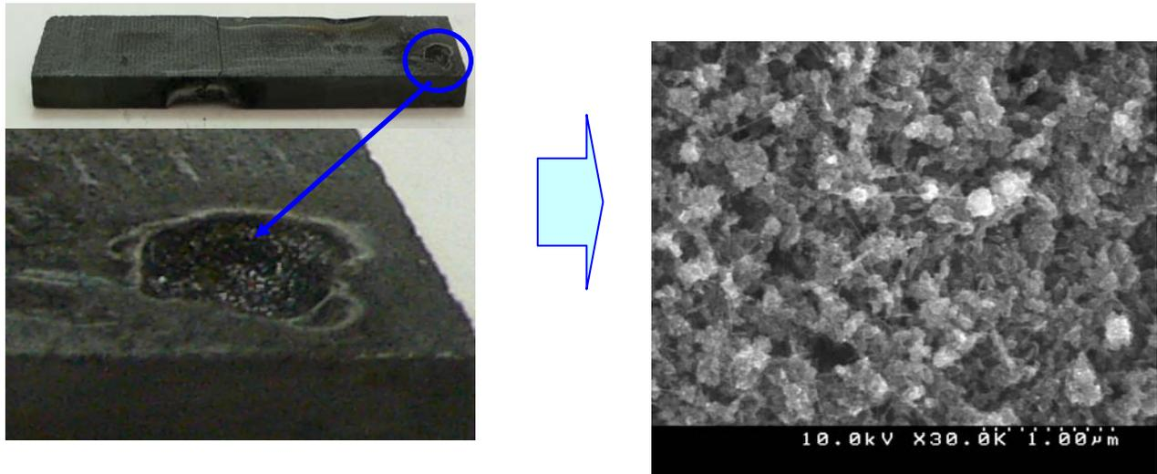
Fig.6 MWCNT observed at the surface of the experiment 5 sample.
