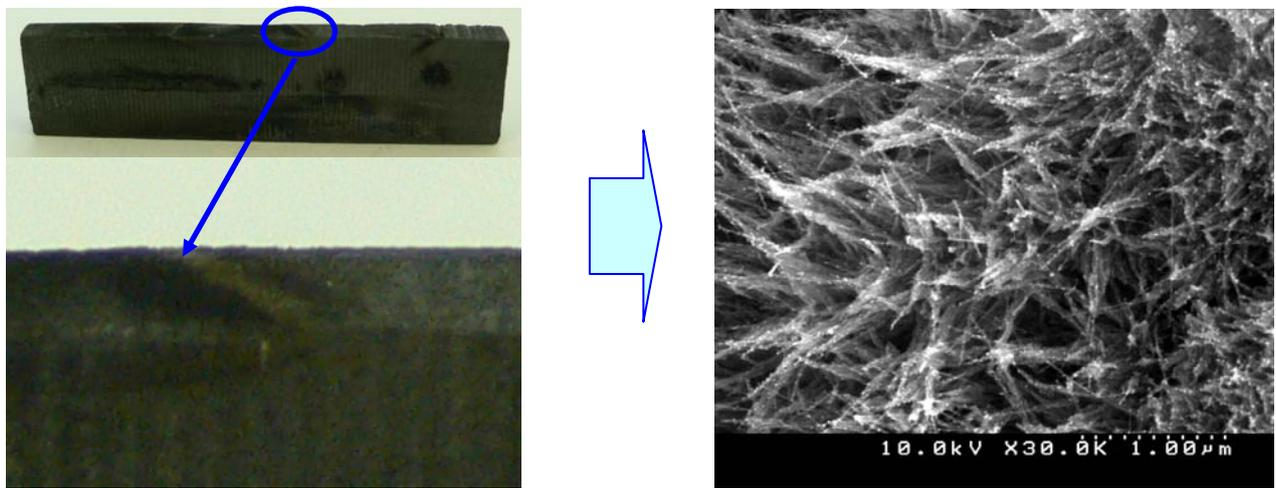
Fig.4 MWCNT observed at the surface of the experiment 3 sample.
