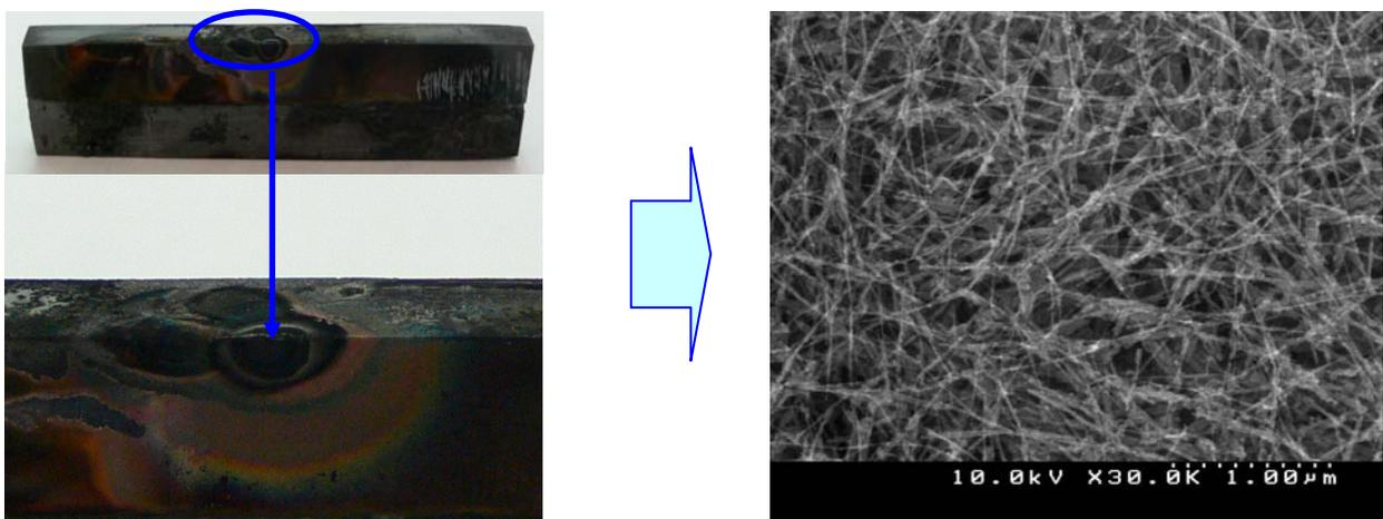
Fig.5 MWCNT observed at the surface of the experiment 4 sample.
