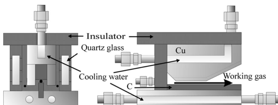
**Fig.1** Schematic diagram of the confront electrode type plasma jet.
