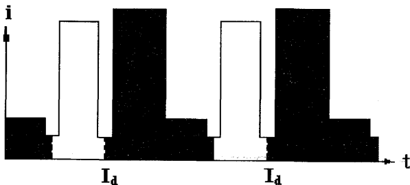
Fig.2 Ideal current waveform for CO 2 arc welding
