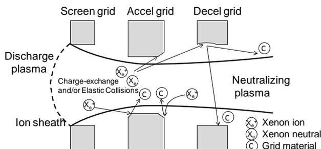
**Fig. 1** Grid erosion mechanism in ion engines.
