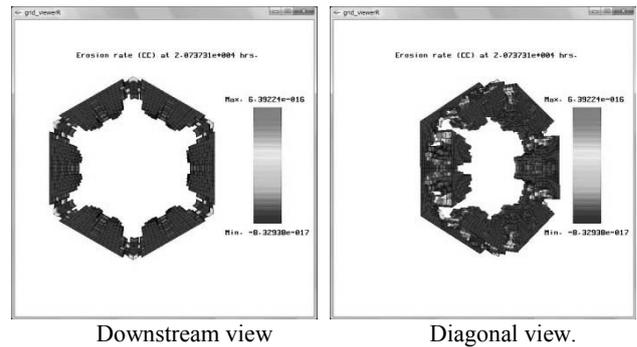
**Fig. 5 (b)** Decel grid after 20,000 h of operation for  $\phi_a = -350$  V.
