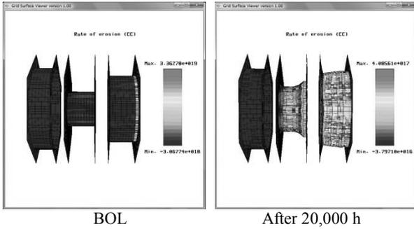
**Fig. 3 (a)** Grid surfaces and erosion intensities in the high beam current region for  $\phi_a = -350$  V.
