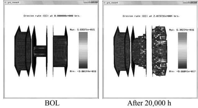
**Fig. 5 (a)** Grid surfaces and erosion intensities in the low beam current region for  $\phi_a = -350$  V.
