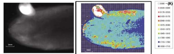
Fig. 9 Weld pool temperature in CO<sub>2</sub> arc welding.
