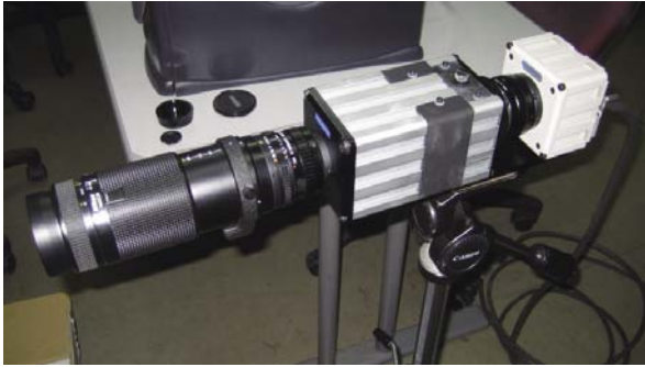
Fig. 3 Photograph of high-speed temperature measurement system by two-color pyrometry.
