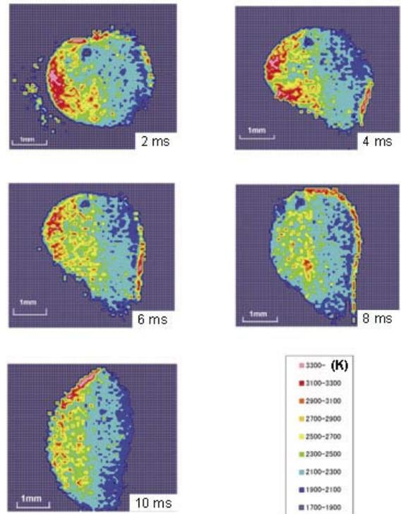
Fig. 6 Time variation in droplet temperature in CO<sub>2</sub> arc welding.
