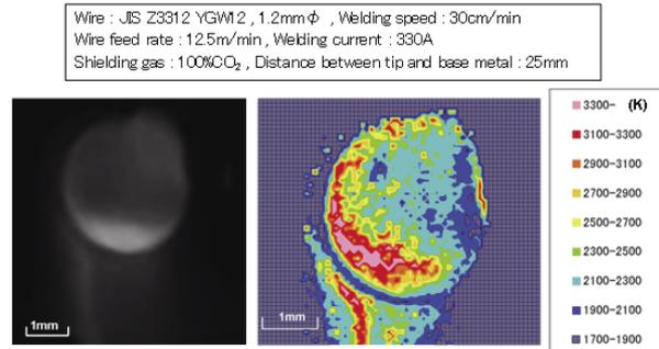
Fig. 5 Droplet temperature in CO<sub>2</sub> arc welding.
