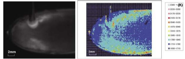
Fig. 8 Weld pool temperature in MAG welding.
