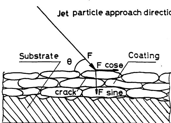
Fig. 12 Schematic diagram of cross-section structure of coating and interaction between coating and jet particle.
