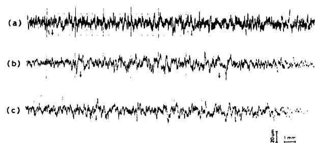
Fig. 5 Surface roughness curves of TiO<sub>2</sub> coatings: (a) as sprayed surface, (b) the same surface as Fig. 4 (e), (c) the same surface as Fig. 4 (f).
