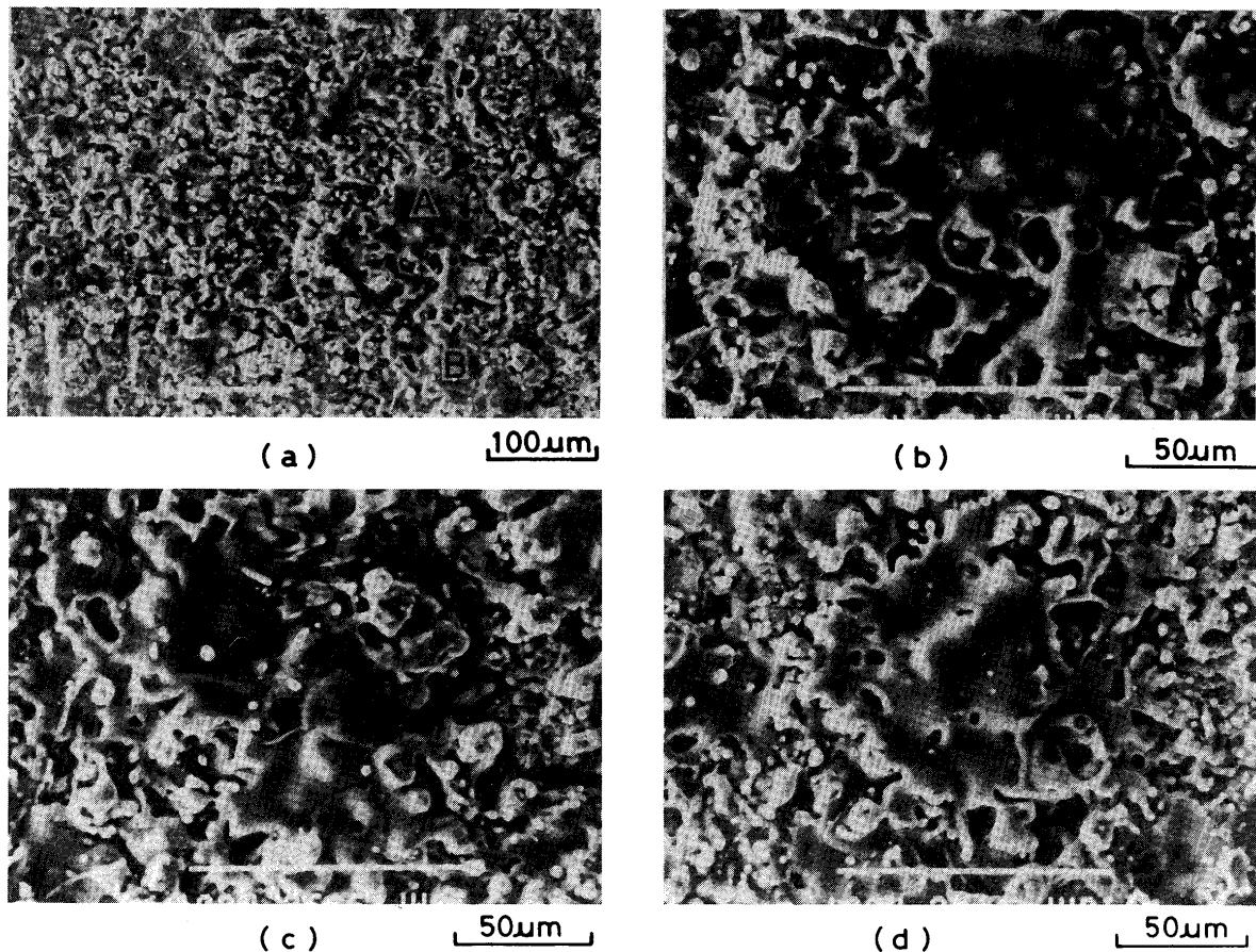
Fig. 9 SEM photographs of as sprayed coating surface of 40% $\text{TiO}_2$  ceramics: (b) and (c) are areas A and B in (a) respectively.
