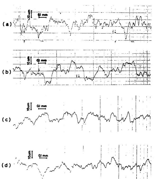
Fig. 8 Comparison of surface roughness of ceramics coatings (cut-off of waveness: 0.8 mm): (a) and (b) are roughness curves before and after ACT-JP test for 40% $\text{TiO}_2$  coatings, (c) and (d) are those before and after ACT-JP test for  $\text{Al}_2\text{O}_3$  coating respectively.
