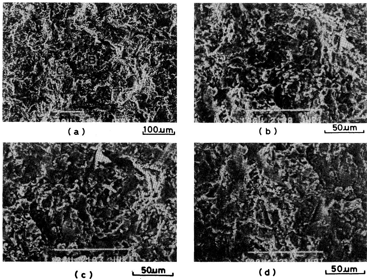
Fig. 10 SEM photographs of 40% $\text{TiO}_2$  coating surface after ACT-JP test; (b), (c) and (d) are areas A, B, C in (a) respectively.
