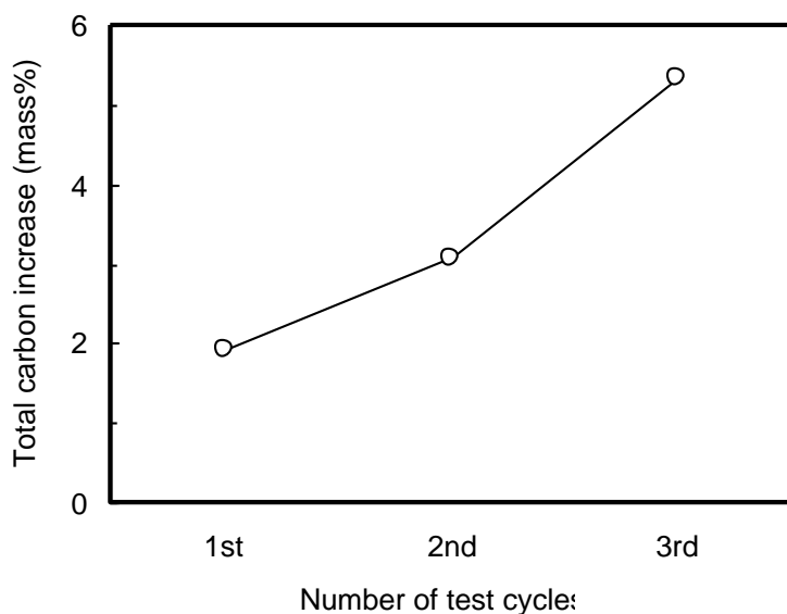
Figure 3-4 Total carbon increase of alloy A as a function of test cycles. Data were taken for the specimens right after exposure to a 15%CH 4 -3%CO 2 -82%H 2 gas mixture at 1,100°C for 96h.
