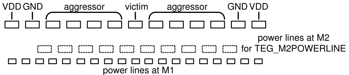
Figure 2.15: Interconnect structure for RLC extraction.
