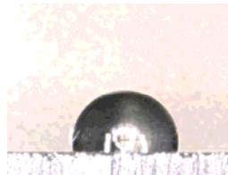
(ii) 撥水処理後 ( \theta = 104^\circ )
