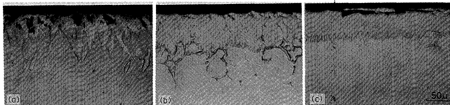
Fig. 8 Crosssectional microstructures of iron and nickel group after treatment of 950°C, 3 hrs: (a) Fe, (b) Fe-36%Ni, (c) Ni (as-polished).
