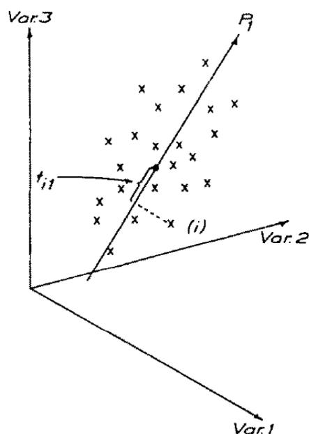
**Figure 2.2.** A data matrix  $\mathbf{X}$  is represented as a swarm with  $N$  points in a  $K$ -dimensional space. This figure shows a 3-space with a straight line fitted to the points: a one-component PC model. The PC score of an object ( $t_i$ ) is its orthogonal projection on the PC line. The direction coefficients of the line from the loading vector  $p_k$ . [27]
