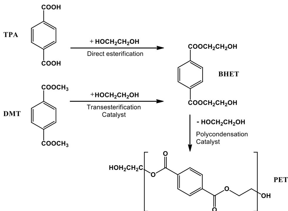
**Scheme 1.2.** Schemes for the PET polymerization process. [1]
