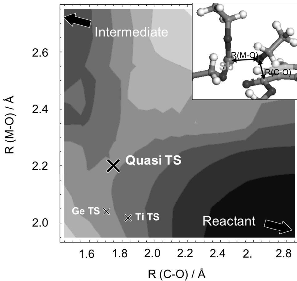
**Figure 3.7.** Contour plot of the potential energy surface of the  $\text{Sb}(\text{OEt})_3$  catalyzed reaction in the coordination of carbonyl oxygen atom mechanism. TS geometries for  $\text{Ge}(\text{OEt})_4$  and  $\text{Ti}(\text{OEt})_4$  catalysts are also indicated.
