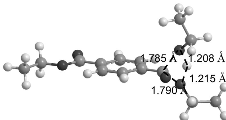
**Figure 3.2.** Optimized structure for the TS complex of transesterification reaction of DET with ethanol without catalyst. Reaction path with four-centered TS was assumed.
