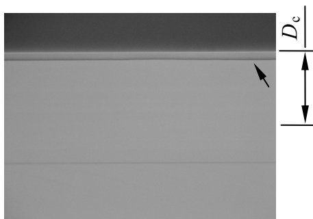
(b) Belt-shaped mark of the laser scribed crack surface generated by laser overlapping irradiation ( P_2 = 91.5 \text{ W} , v_2 = 300 \text{ mm/s} )
