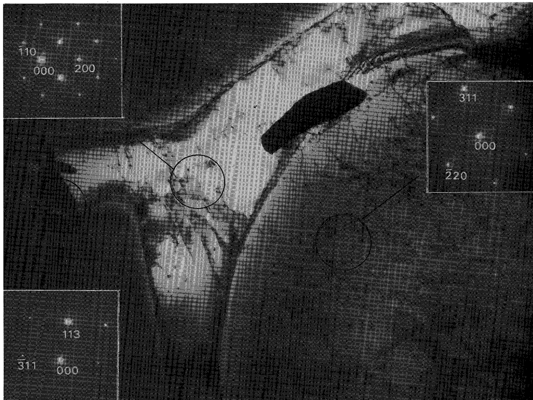
Photo. 2 (A) Transmission electron micrograph of overlaying stainless steel, showing a ferrite grain, NbC and M_{23}C_6 type carbides. (36000 \times 4/5)
