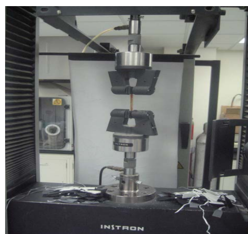
Fig. 9 Clay/polymer nanocomposite sample during mechanical test.
