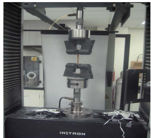
Fig. 9 Clay/polymer nanocomposite sample during mechanical test.
