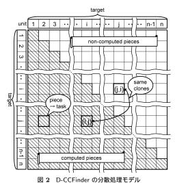
Fig. 2 Distributed processing model of D-CCFinder.
