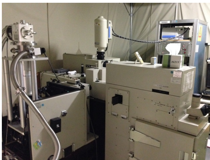
Figure 4.15: The Raman system triple-grating T64000 at S. TAJIMA group in OSAKA University.
