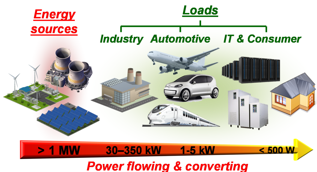
Fig. 1-1 Applications of power electronics with approximate power ratings
