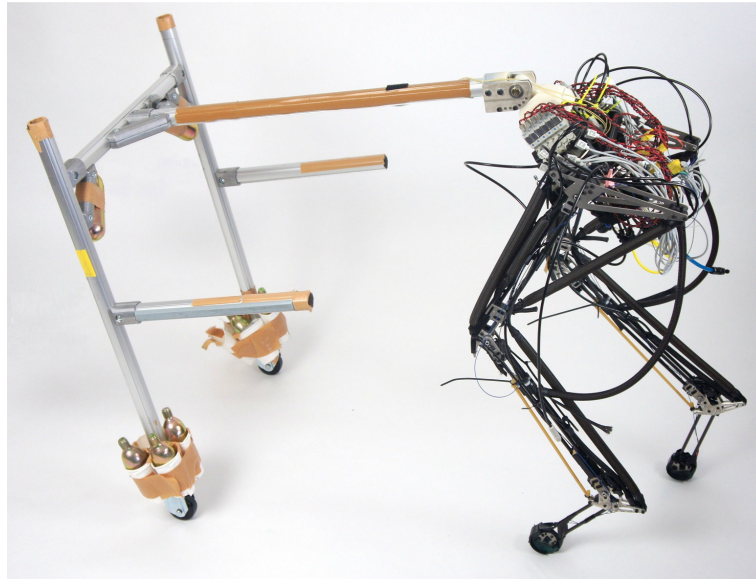
Figure 4.1: The robot possess hindlimb dimensions similar to a cheetah, with realistic moment arms to produce scientifically relevant locomotion during EMG-based muscular activation.
