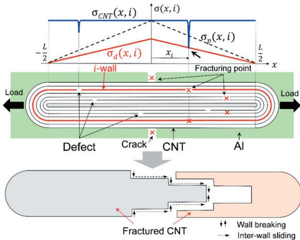
**Fig. 5** Scheme of stress distribution on a wall of MWCNT and the peeling fracture mode of MWCNT during tensile failure.
