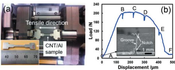
**Fig. 1** Tensile stage placed in SEM (a) and recorded load-displacement curve for in-situ observation of CNT/Al composite during the tensile test (b).
