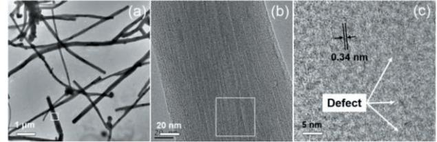
**Fig. 2** Morphology of raw MWCNT by TEM observations at different magnifications. (b) shows the box in (a). (c) shows the box in (b).
