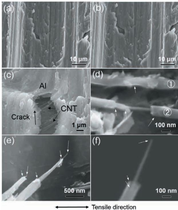
**Fig. 4** In-situ SEM observations of CNT during different processes in tensile test. (a) through (f) are corresponding to the states in Fig. 1b. White arrows in (d) through (f) indicate the positions of vertical wall-breaking. Longer arrows suggests the later happened breaking for each CNT.
