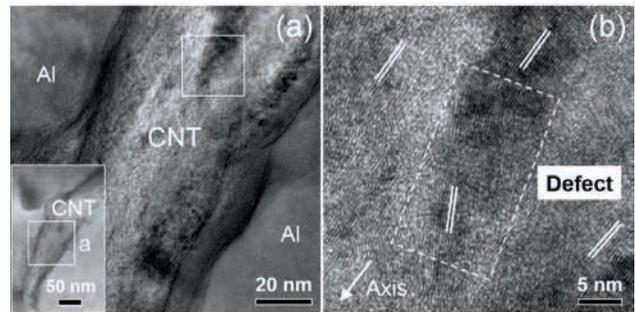
**Fig. 3** Morphology of MWCNT dispersed in AMCs by TEM observation at different magnifications. (b) shows the box in (a). Double-lines in (b) suggest the aligning direction of walls.
