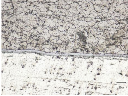
Fig. 2 Optical microstructure near welded interface
