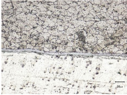
Fig. 2 Optical microstructure near welded interface
