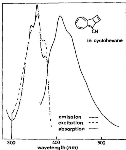
Fig.11 Abs. Fluor. and Excit. Spectra of (1) in cyclohexane
