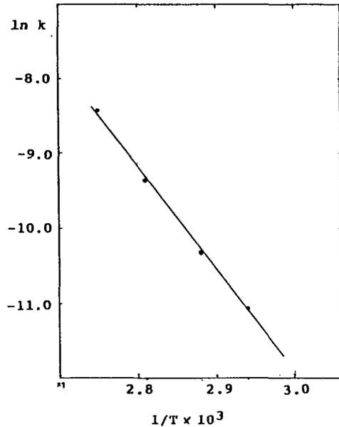
Fig.24 Arrhenius plot for the thermolysis of (2)
