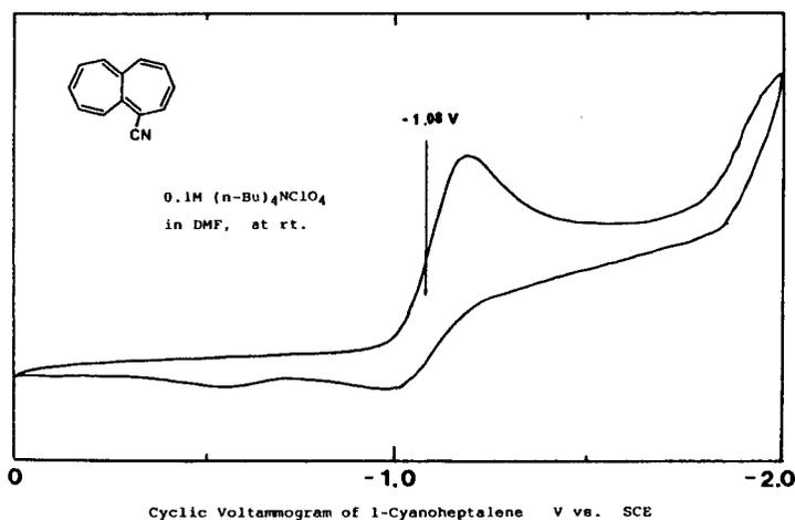
Fig.7 CV of (3) in DMF at 25 °C [ 0.1M  $n\text{-Bu}_4\text{NClO}_4$  as the supporting electrolyte ]
