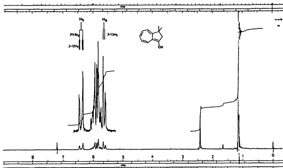
Fig.14 100MHz <sup>1</sup>H-NMR Spectrum of (9) in CDCl<sub>3</sub>
