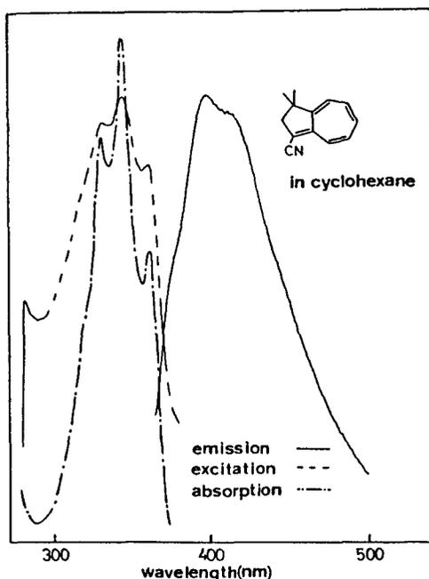
Fig.15 Abs. Fluor. and Excit. Spectra of (9)
