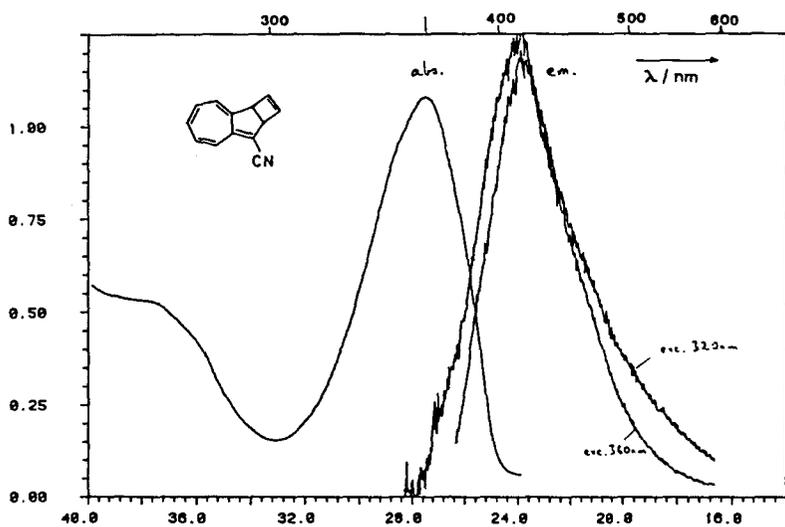
Fig.13 Abs. and Fluor. Spectra of (1) in MeOH
