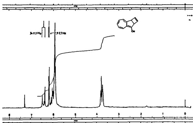
Fig.1 100MHz  $^1\text{H-NMR}$  Spectrum of (1) in  $\text{CDCl}_3$
