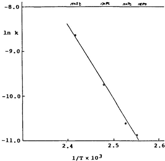
Fig.23 Arrhenius plot for the thermolysis of (1)
